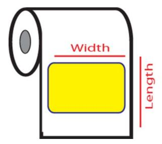
Label Repeat: the measurement from the top of one label to the top of the next label.
